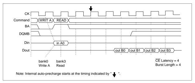
Write with Auto Precharge to Read Command Interval (Different bank)
