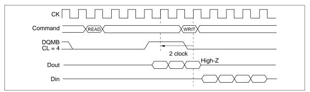
**2. Same bank, different ROW address:** When the ROW address changes, consecutive write commands cannot be executed; it is necessary to separate the two commands with a precharge command and a bank-active command.
