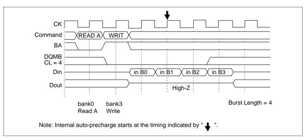
Read with Auto Precharge to Write Command Interval (Different bank)
